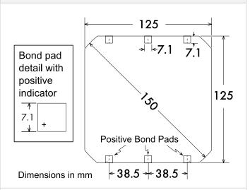
Bond pad area dimensions are  $7.1\,\mathrm{mm} \times 7.1\,\mathrm{mm}$ Positive pole bond pad side has "+" indicator on leftmost and rightmost bond pads.
